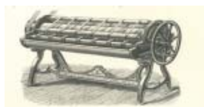
Sheet-fed wetting machine - from Gaskell 1877
